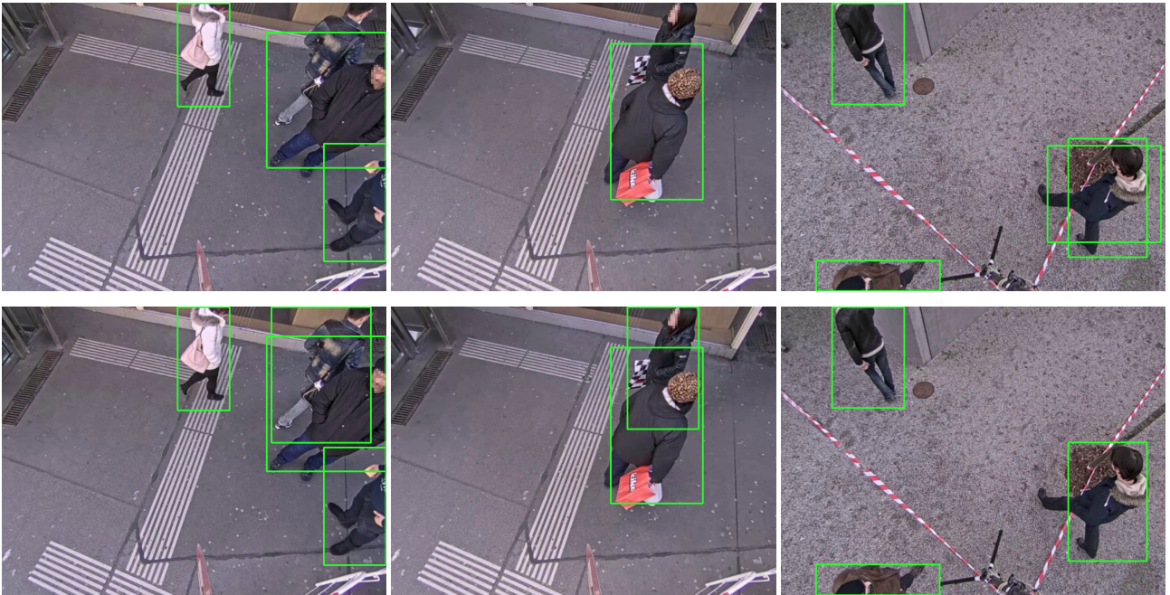
Figure 6: Qualitative comparison of the best performing greedy NMS threshold (first row) and Tnet (second row). Both models operate on the same precision. Selecting a fixed greedy NMS threshold leads to missed detections (first two columns) and multiple detections for a single person (rightmost column), whereas our modified Tnet is able to cope with such scenarios.
